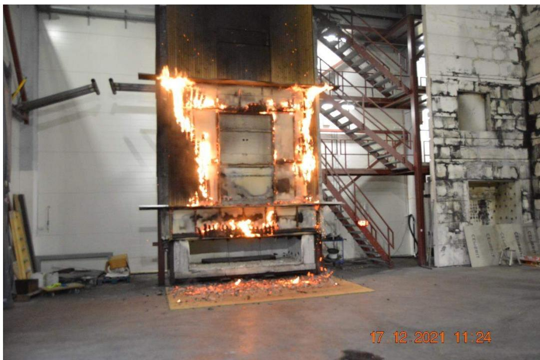
Photo No. 18 Test specimen approximately 25 minutes after the heptane burned out.
