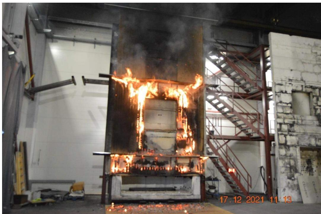
Photo No. 16 Test specimen approximately 14 minutes after the heptane burned out.
