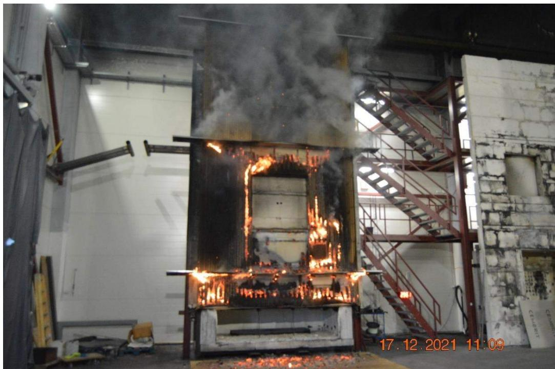
Photo No. 15 Test specimen approximately 10 minutes after the heptane burned out.
