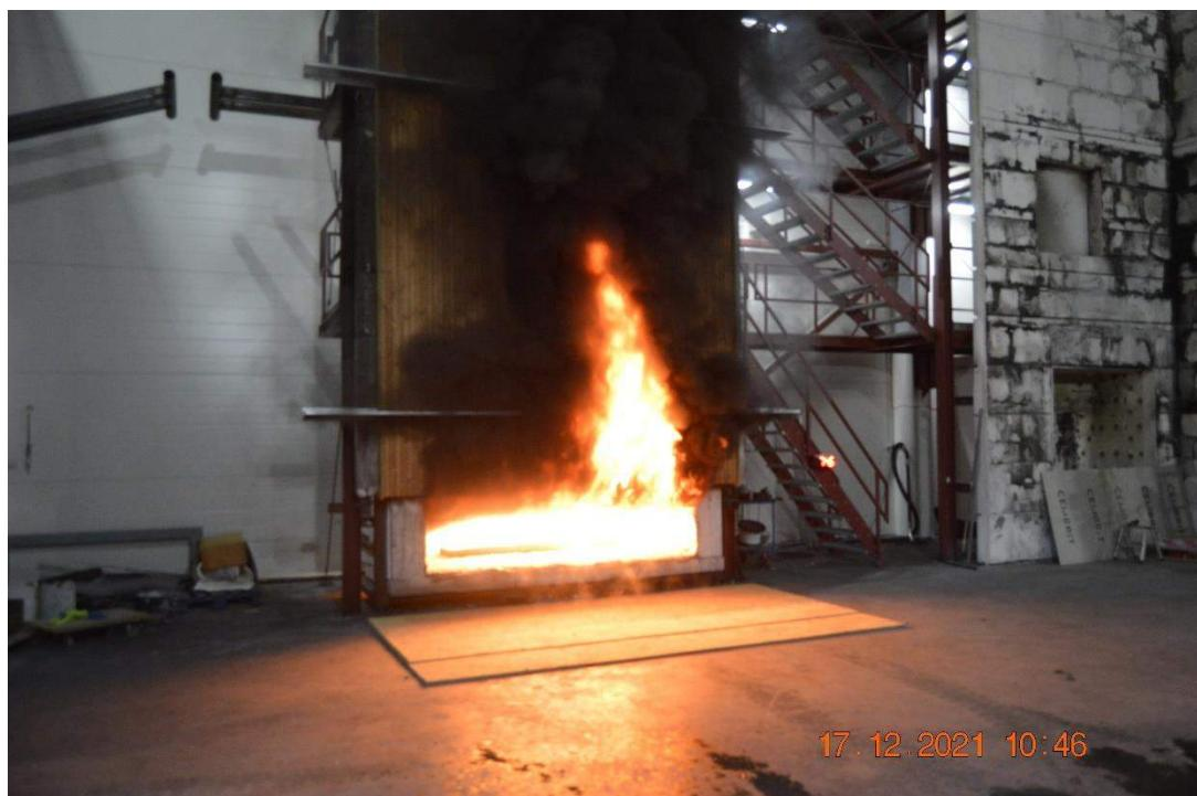
Photo No. 10 Test specimen after 7 minutes of testing
