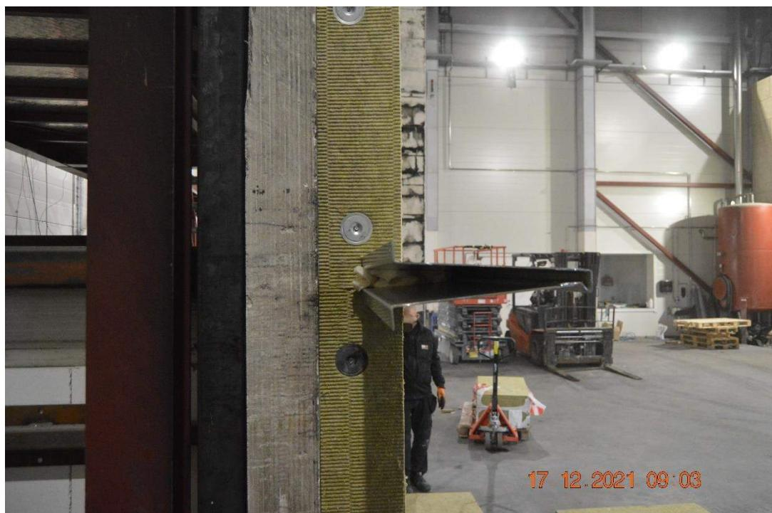
Photo No. 8 First fire screen with insulated edge of the wall
