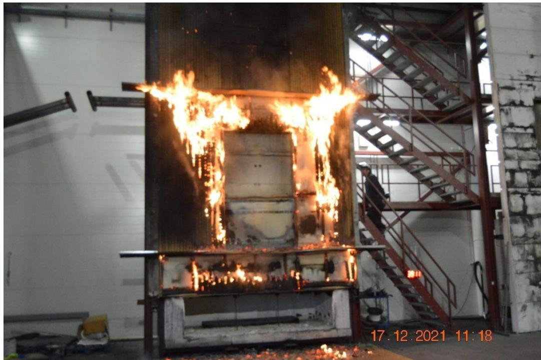
Photo No. 17 Test specimen approximately 19 minutes after the heptane burned out.
