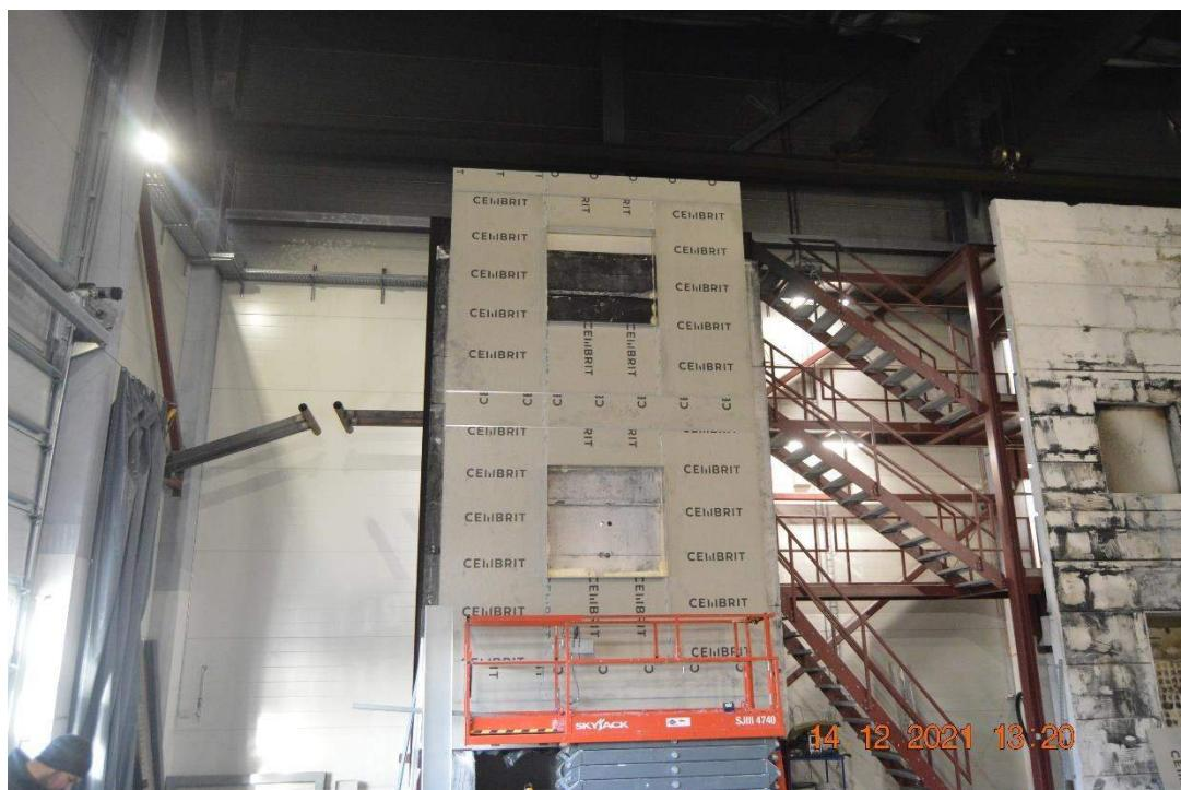
Photo No. 4 Cembrit boards and steel profiles around windows mounted
